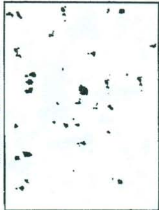
Rust Grade 8-G, 1% Rusted
