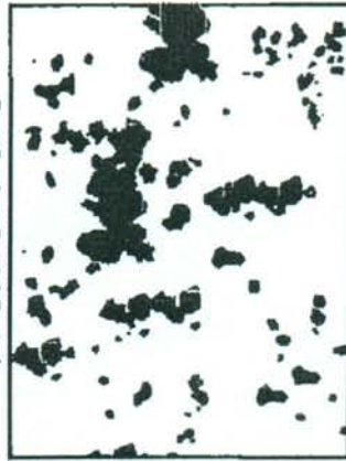
Rust Grade 3-G, 16% Rusted
