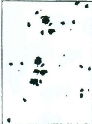
Rust Grade 5-G, 3% Rusted
