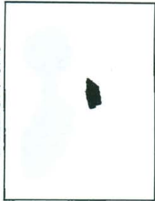
Rust Grade 6-S, 1% Rusted
