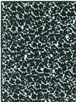
Rust Grade 1-P, 50% Rusted
