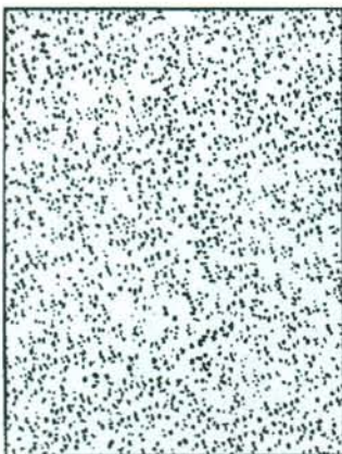
Rust Grade 4-P, 10% Rusted
