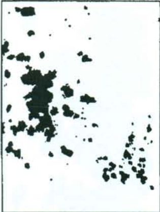
Rust Grade 4-G, 10% Rusted FIG. 2
